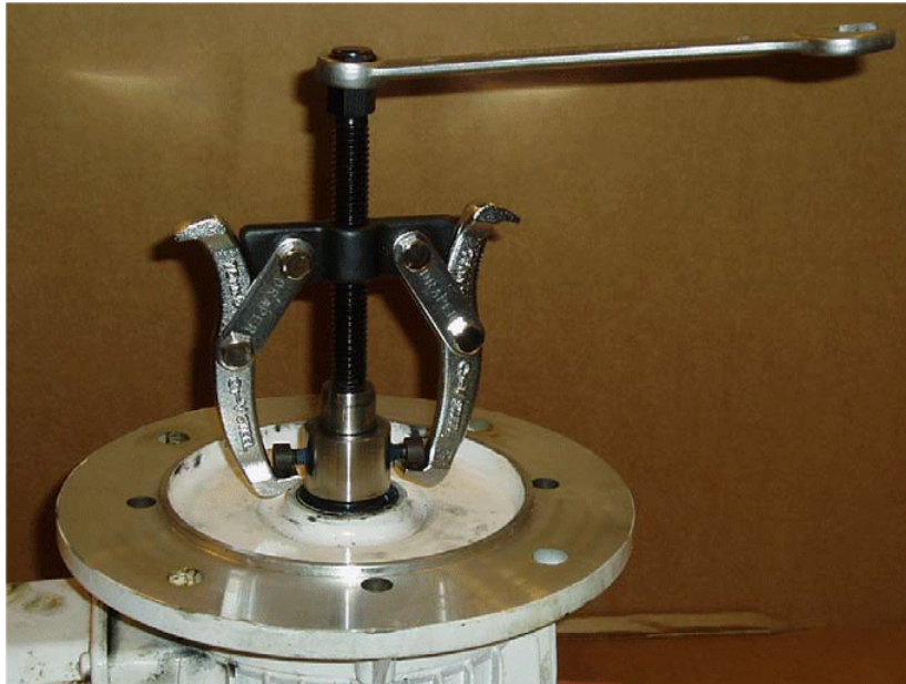
Figure 5.31 Removing Rehffuss coupling hub using Two Leg Puller
